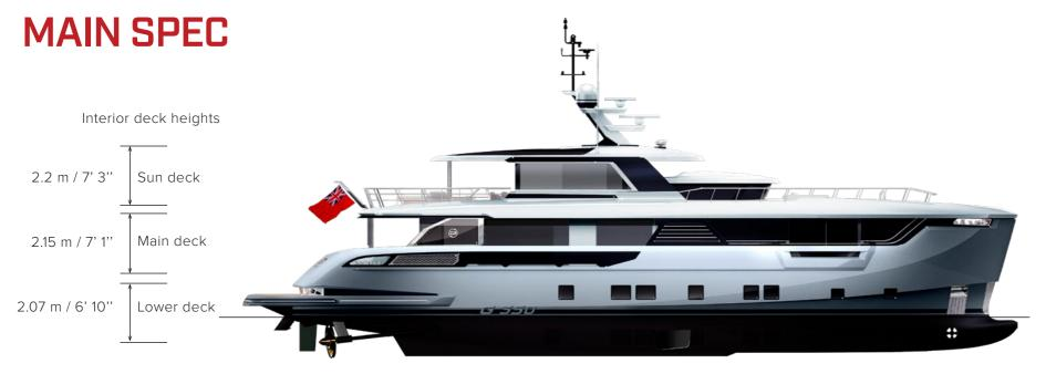
Length overall:34.7 m / 114'Beam:8.5 m / 27' 1"Draft:1.8 m 4' 11"Material:Aluminium / SealiumHull type:Round bilge, fast displacementTonnage:299 GT
